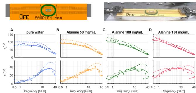
**Fig. 3.** **Up** The designed chip. **Down** Real and imaginary parts of relative complex permittivity of a liquid specimen obtained using our chip (circles) vs. reference coaxial probe bulk measurement (solid line) and from molecular dynamics simulation (dashed line) for A) pure water, B) 50 mg/mL, C) 100 mg/mL, and D) 150 mg/mL of alanine concentration in the water. Adapted from [4].
